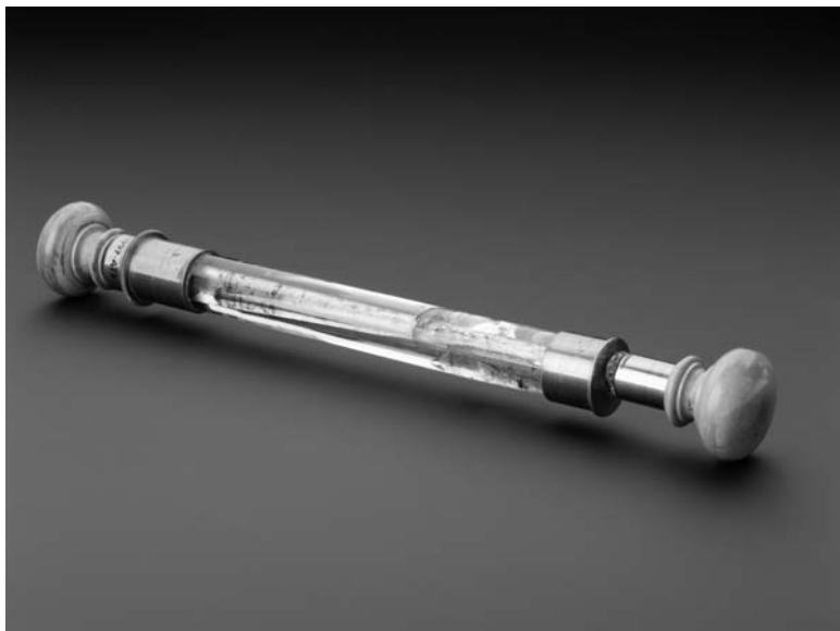
Fig. 10.3 A French demonstration model of a fire piston, early nineteenth century (Science Museum, London/SSPL).
