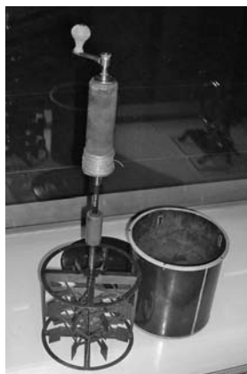
Fig. 14.2 Joule's paddle-wheel calorimeter, 1845 (Science Museum, London/SSPL).
