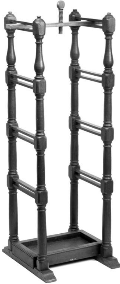
Fig. 7.1 Poleni's apparatus (similar to 's Gravesande's) for free fall into clay (photograph from the Boerhaave Museum, Leiden).
